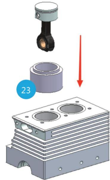
The piston ring and cylinder liner shall be matched one by one, and then installed in the corresponding cylinder liner
